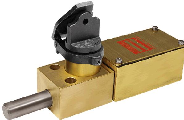
Type S auxiliary switches are slow-make, slow-break devices that respond directly to the movement of the lock bolt when the key is rotated. One, two, three or four sets of contacts are available. The Type S auxiliary switches can be furnished on the following interlocks:
